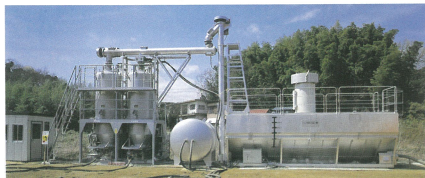
改良材供給機(左)と改良材サイロ(右) Agent feeder(left), Agent silo(right)
