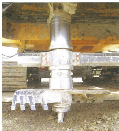
攪拌翼(土研式) Mixing blade (Standard type)
