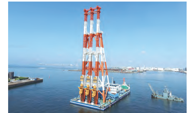
Vessel for offshore ground improvement work: Pioneer 30 Fudomaru sand compaction vessel
