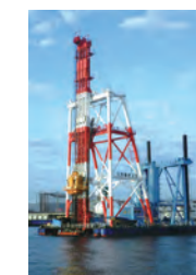
Vessel for offshore ground improvement: Deep mixing process vessel Fudo No. 7
